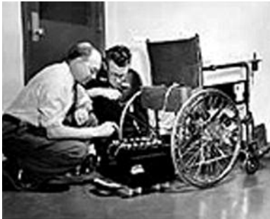
The NRC's George Klein and Robert Owens at work on the prototype electric wheelchair, in the early 1950s. The prototype can be seen at the Canada Science and Technology Museum in Ottawa.
